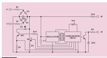
Fig.11 Schematic diagram - XP95 Heat detector
